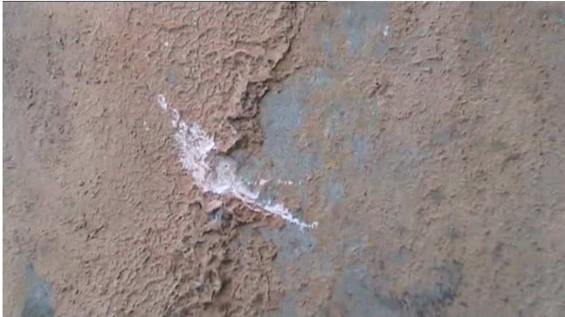
Figure 126. Brown mineralisation chipped but largely resistant to removal
