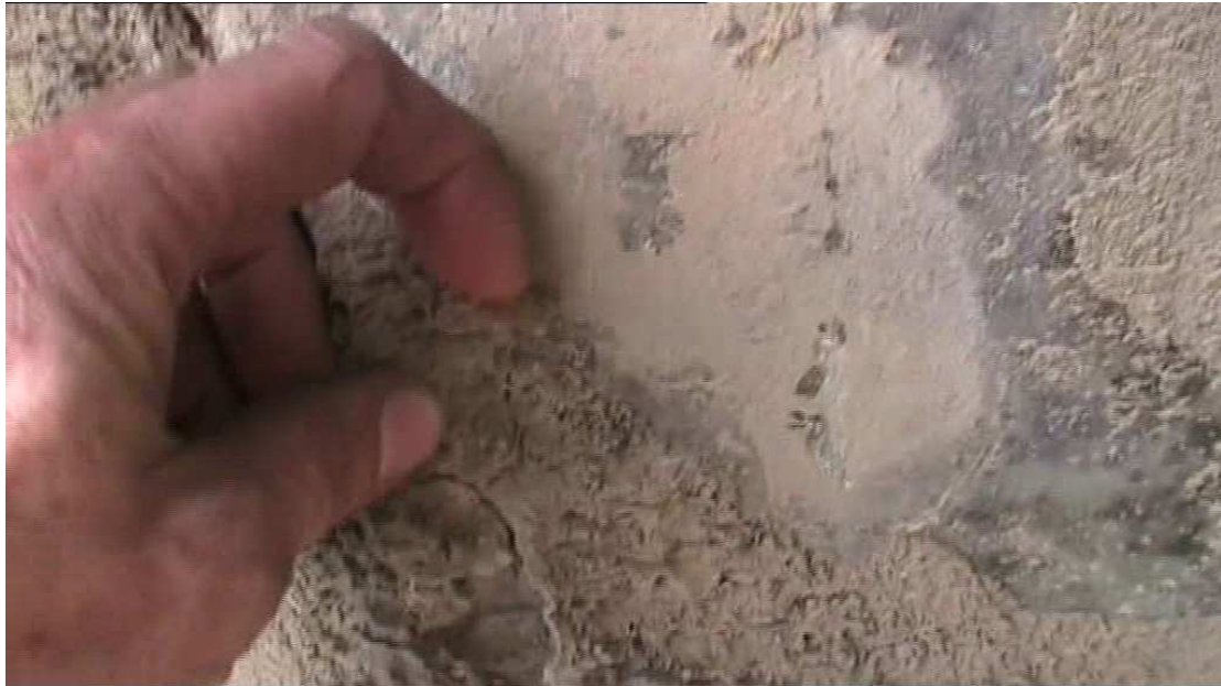
Figure 136. Testing brown mineralisation for adhesion by hand
