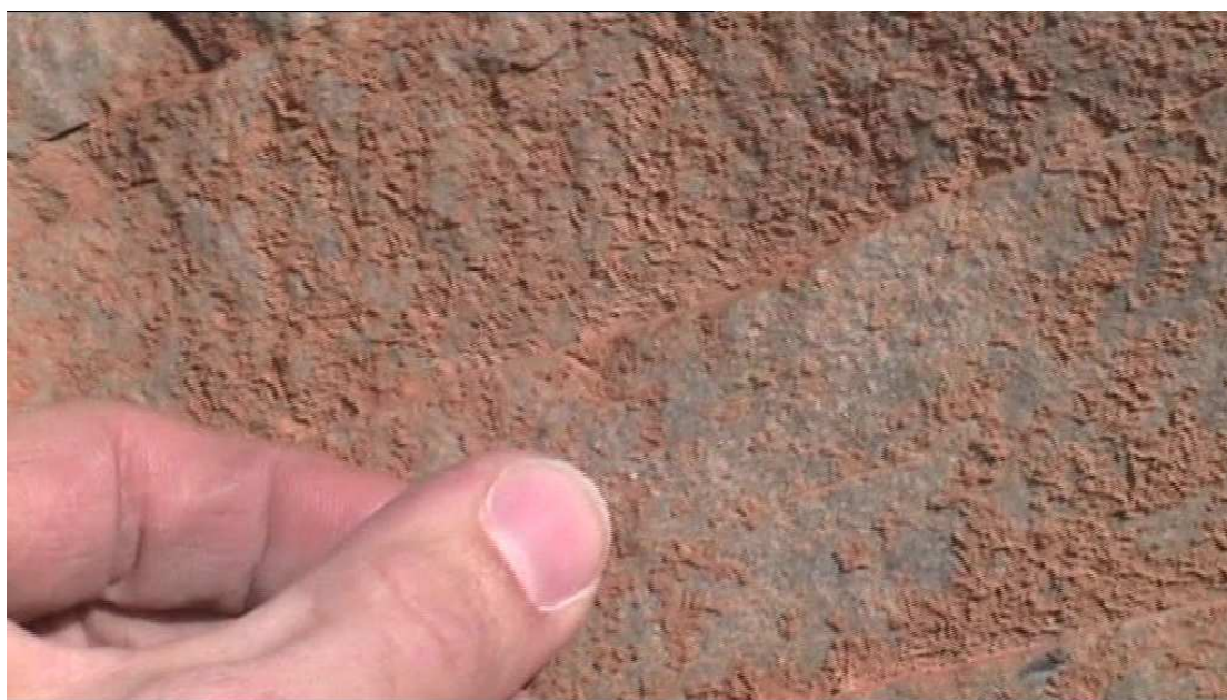
Figure 111. Testing brown mineralisation for adhesion by hand
