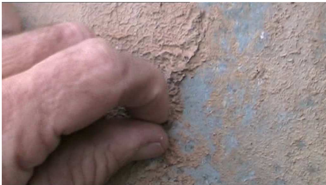
Figure 124. Testing brown mineralisation for adhesion by hand
