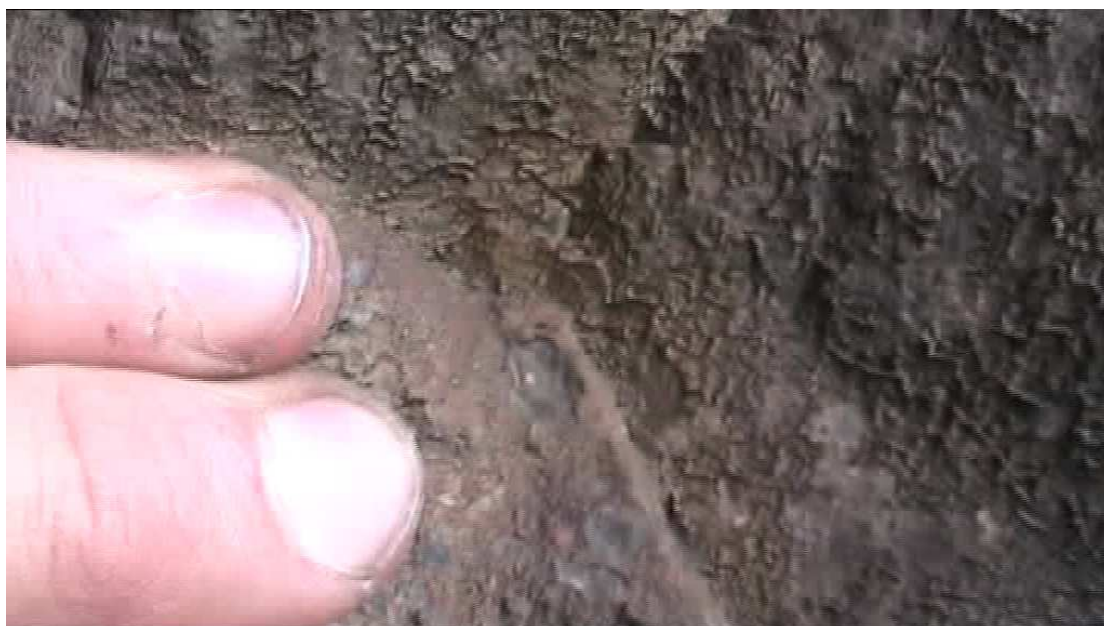
Figure 118. Testing brown mineralisation for adhesion by hand
