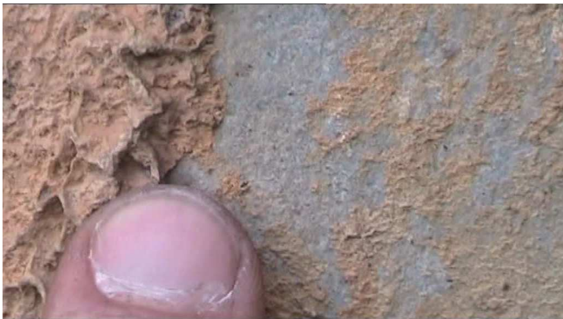
Figure 123. Testing brown mineralisation for adhesion by hand
