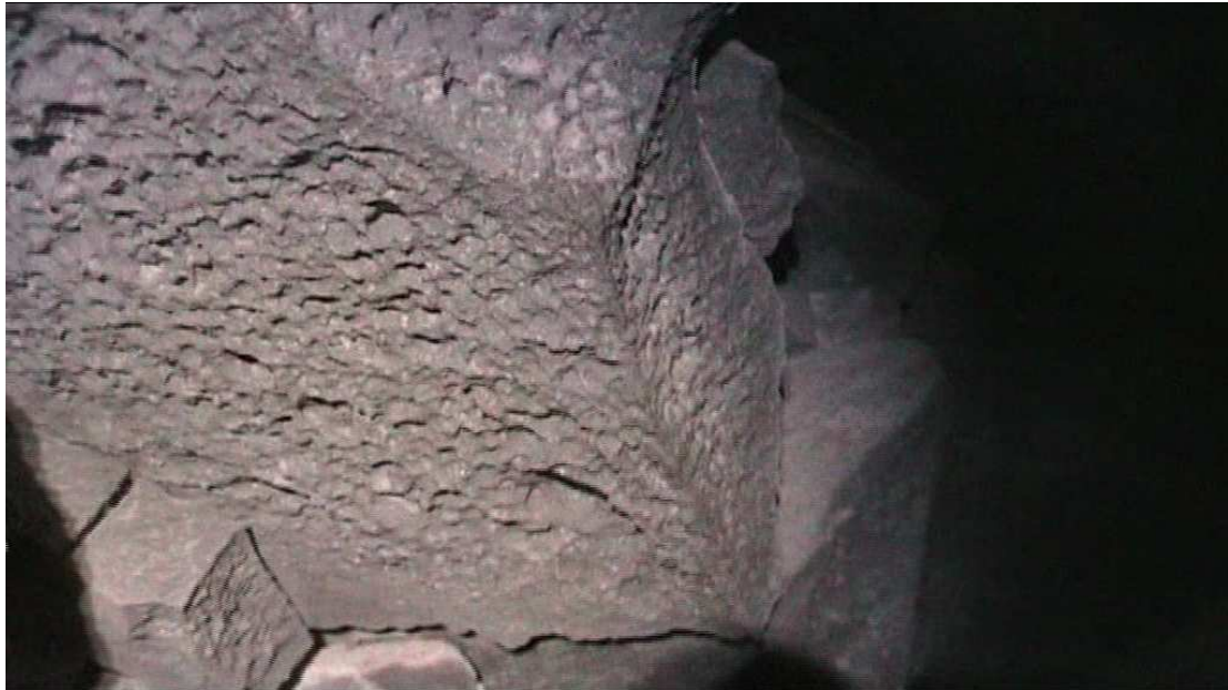
Figure 161. Hard, mineralised rock with pock marked erosion patterns
