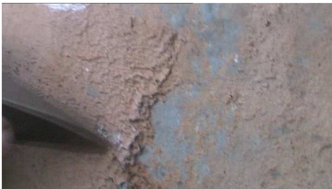
Figure 125. Testing brown mineralisation for adhesion by use of a tool
