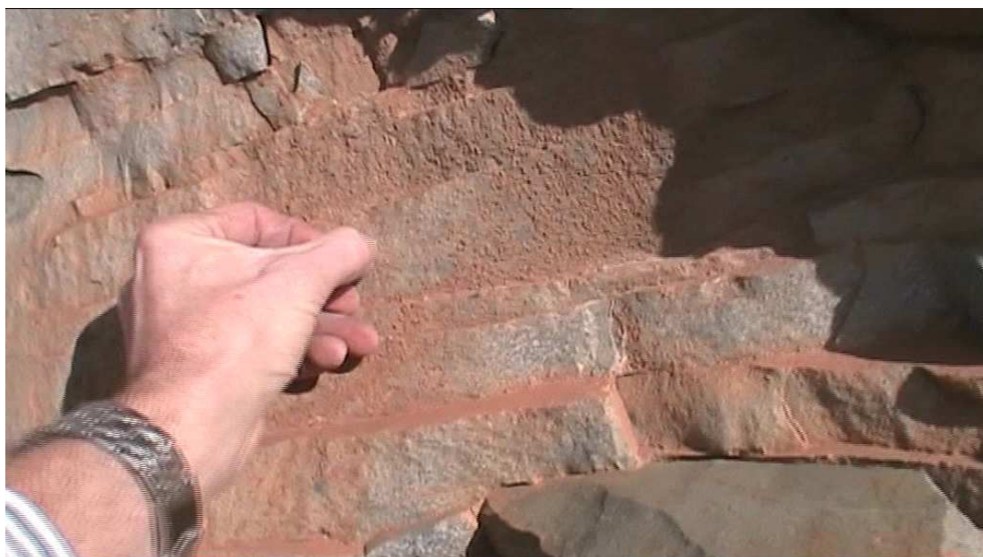
Figure 110. Testing brown mineralisation for adhesion by hand
