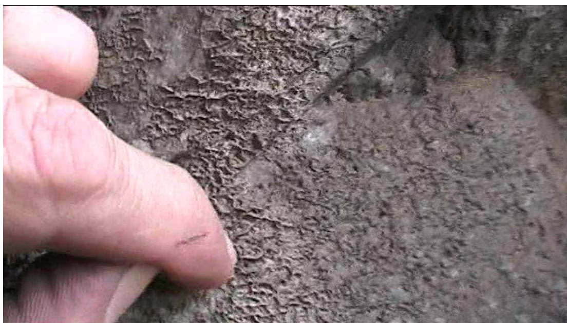
Figure 117. Testing brown mineralisation for adhesion by hand
